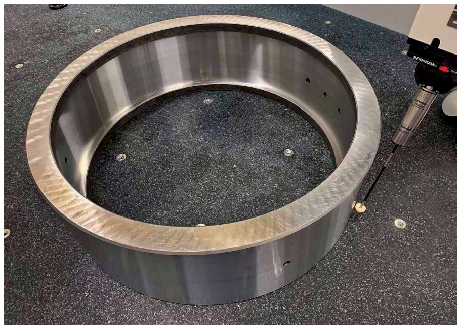
— Bearing outer race inspection in progress by touch probing and scanning in a single 10-minute cycle.
