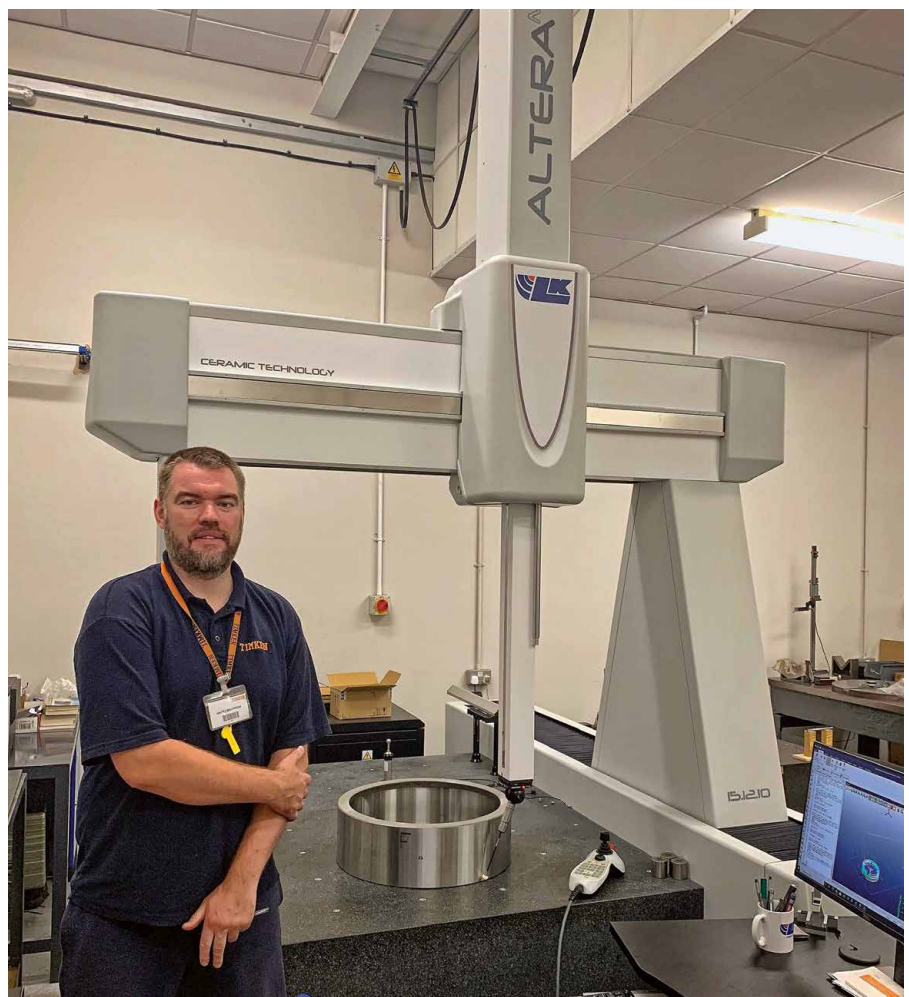
—William Hayes, Quality Improvement Engineer at the Dudley factory of The Timken Company, with the new LK Metrology AlteraM 15.12.10 ceramic bridge coordinate measuring machine.
