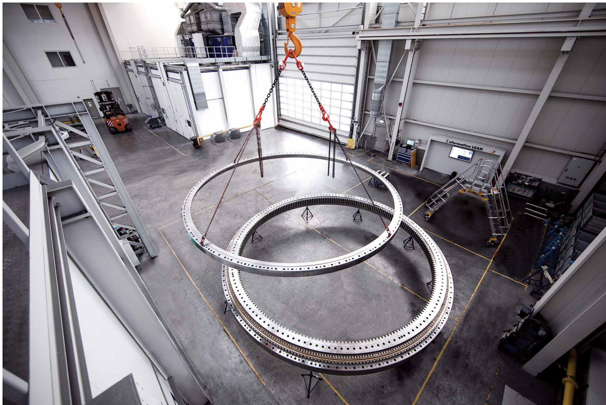
—When two become one: The retaining and the support rings are precisely placed on top of each other.
