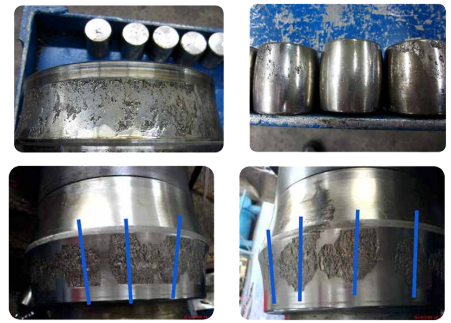
— Fig. 10: Potentially harmful situations. Surface distress/wear despite good lubrication.
