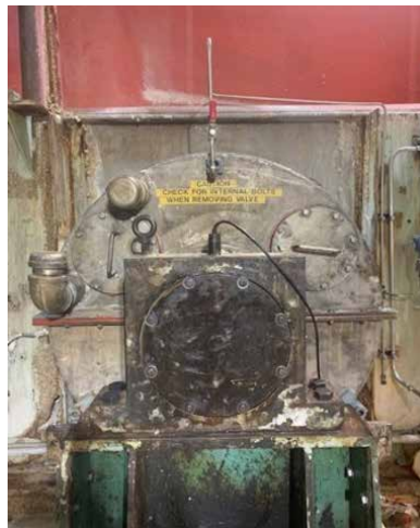
— Bleach decker with the ultrasonic sensor mounted on the bearing
