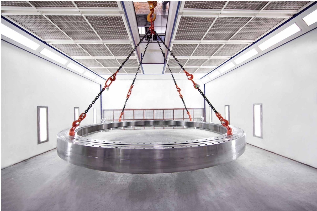
— The finishing touch: The slewing bearing is preserved, so that it safely reaches China.
